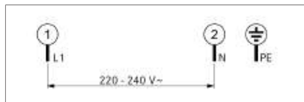
Fig. 4.44 Connection diagram 1-phase connection cooktop
